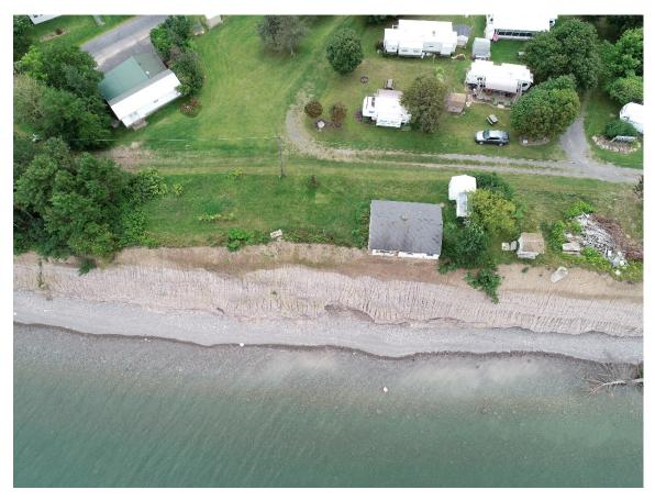
Figure 2-3 Undermined Structures
