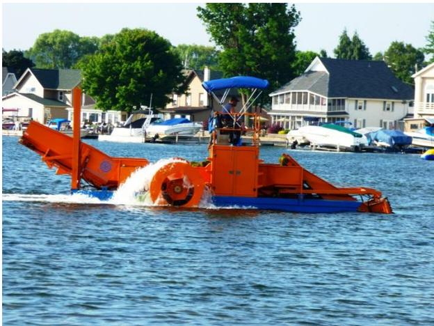
Non-harvesting down time due to mechanical issues and repairs was significantly reduced this season. This was primarily due to the program having the most up to date equipment it has seen in a while. Maintenance issues were mostly related to the moving parts systems of the harvesters' cutting head (i.e. broken/bent knives, worn out tie-rod bearing). The operating crew and crew leader make a superb effort to return the harvesters to operation as soon as possible when mechanical issues arise.
