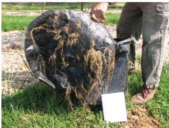
**Figure 19. Ash roots penetrating geotextile after compacted subsoil has been washed away. Roots increased infiltration by a factor of 27.**
