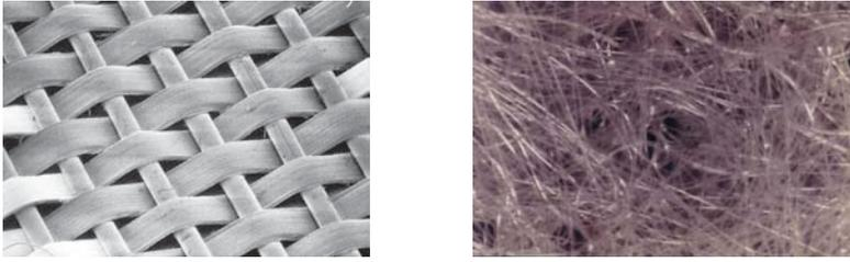
**Figure 9. Enlarged view of woven and nonwoven geotextiles.**
