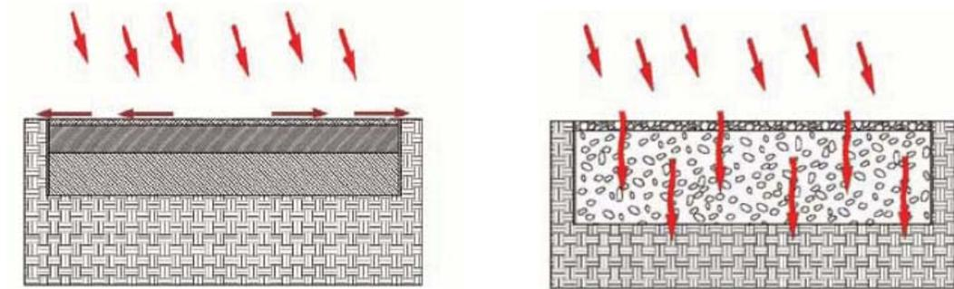
**Figure 17. The left figure shows rain on a traditional asphalt parking lot- after it hits the surface it typically runs off into a storm sewer system. The right figure shows rain on a porous asphalt parking lot- after it hits the surface it infiltrates through the pavement into the structural soil reservoir below. Water then infiltrates into the ground, recharging the groundwater over time.**
