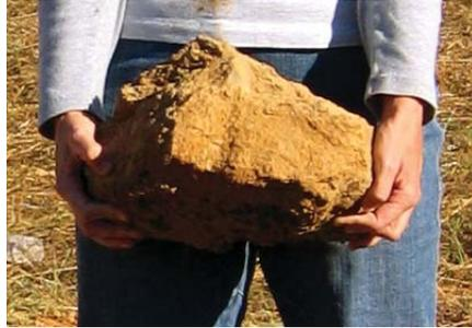
**Figure 5. Compacted soil from a typical construction site. Lack of structure prohibits root penetration and growth.**
